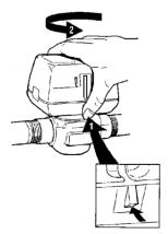
Figure 3: Actuator Head Removal.
