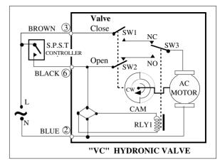
Figure 7: Actuator wiring for SPST controller
