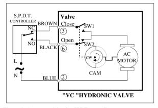
Figure 6: Actuator wiring for SPDT controller
